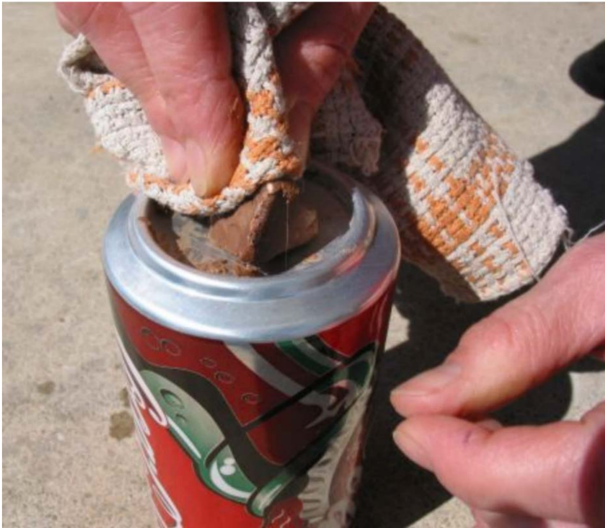
Figure 4 Polishing the Aluminum Can Bottom
