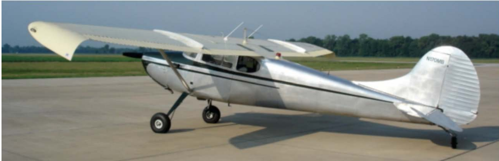
Figure A-8 Drooping the Wing Tips
